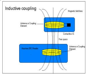
A part of the electromagnetic field generated by the machine (RF) reader covers the antenna of the contactless IC and induces an AC voltage across it. This AC voltage is converted into DC and is used to charge a capacitor. The charge on the capacitor is used to power the IC.
